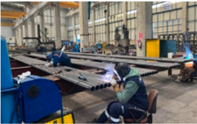
Boiler tube fabrication ongoing in Turkey
