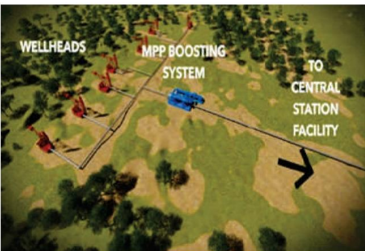
Fig 5: MPP System for Crude Oil Production.
