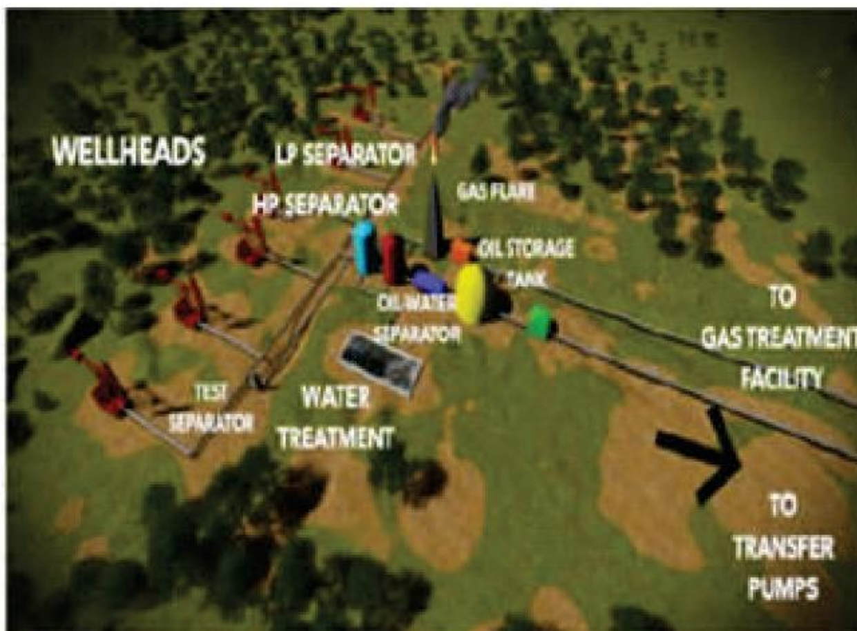
Fig 4: Typical Conventional Production facilities for Crude Oil Production.
